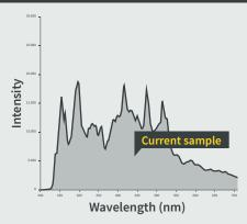
With each measurement, the detector measures the remaining light that has not been absorbed by the measuring medium. This spectrum is also known as the raw spectrum and is stored as intensity *I*.
