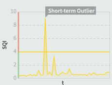
A temporary spike in the SQI can occur as a result of air or particles caught in the measurement path. The Calibration Monitoring feature allows to effortlessly identify short-term outliers and gives the opportunity to ignore measurements exhibiting a higher SQI.
