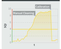
If the SQI remains at an elevated level, even after a manual cleaning, it may be an indication that the current calibration does not cover the water matrix anymore. The issue can be resolved either by improving the existing calibration through the addition of reference values or by creating a new calibration.
