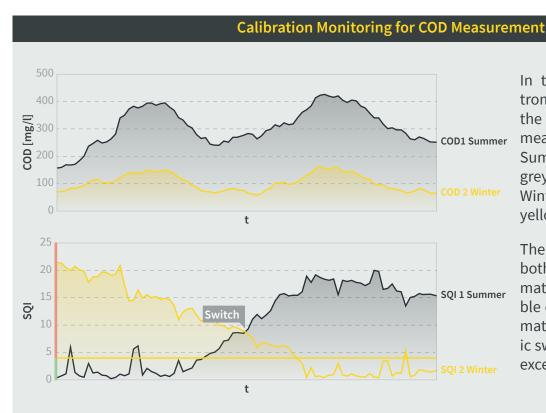
In this example, the UV/Vis Spectrometer simultaneously measures the COD using two calibrations. The measurement values of the COD1 Summer calibration are shown in grey and the values of the COD2 Winter calibration are shown in yellow.
