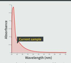
From the clear water calibration and the current raw spectrum, the absorption is finally calculated for each individual wavelength With the calculated values the whole absorption spectrum can be determined.
