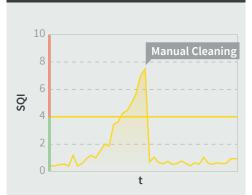
A prolonged exceedance of the SQI threshold value may be an indication for a contamination of the measuring head. In these instances, it is advisable to perform a manual cleaning of the measurement head. If the cleaning resolves the issue the SQI should drop back down to a lower level.
