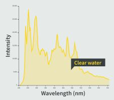
In order to correctly determine the absorption in water, a reference must first be defined. For this purpose, the intensity of the emitted light is recorded for the entire wavelengths in clear water. In order to calculate the ingredients correctly later on, double-distilled water should be used if possible. The clear water spectrum is stored as reference intensity  $I_{\theta}$ .
