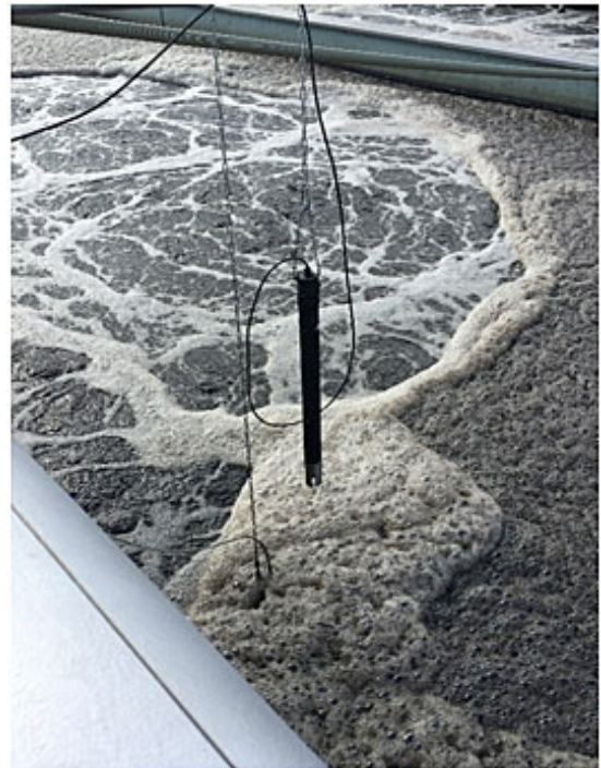
Figure1: GO oxygen sensor in the application of a sewage-treatment plant
